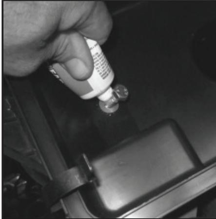
**69** - Install (2) M8 nuts and (2) M8 flat washers to the underside of inner fender mounting plate. Add sealant if needed to insure a water tight seal.
