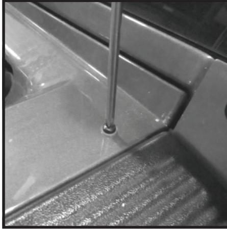
84 - Check alignment of cowl cover and snorkel body. Insert M6 x 20 Phillips head screws to align cover, snorkel and "Z" bracket.
