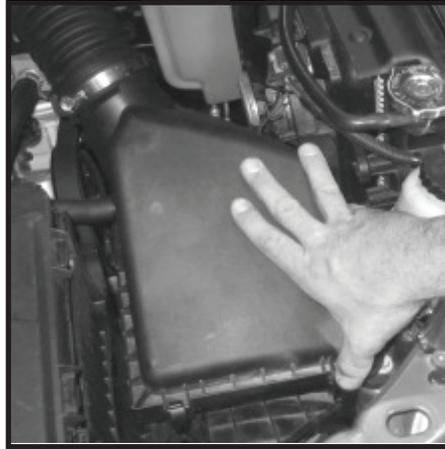
**42 -** Using a flat head screw driver loosen 3" hose clamps at intake and air box. (3.8L shown)
