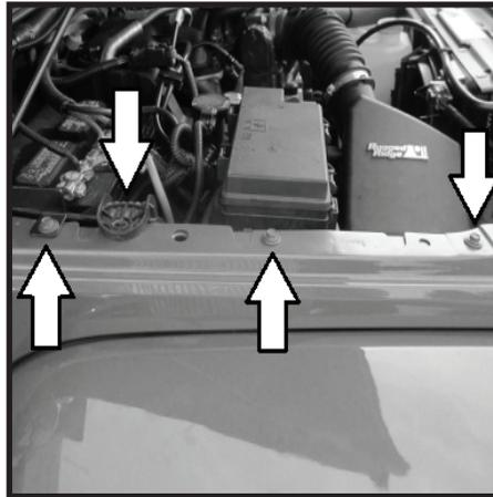
9 - Remove 2 inner cowl bolts located under cowl cover. note location of each bolt. Bolts will be reused.
