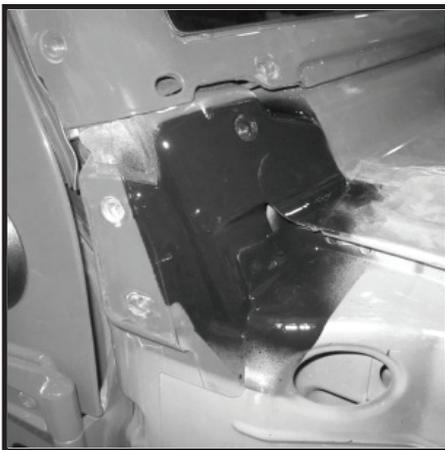
**74** - Reinstall windshield bracket removed in step (2). Start and tighten the upper side M12 bolts and front M12 bolts as shown. Windshield bracket can be adjusted. If needed a screw driver can be used to loosen windshields floating nut plates.
