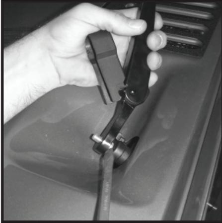
5 - Using a flat head screw driver carefully remove cowl center plastic retainer clips.
