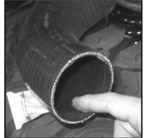
61 - Reinstall 90 deg elbow to lower air box. Align marks made in step (59). Slide 3" clamp onto elbow. With elbow placed against bottom face of lower air box tighten 3" clamp. Pull on elbow to insure it is secured tightly to inlet.
