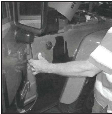
**102** - Align inner door fender tabs with door bolts. Slide tabs under bolts and secure but do not tighten at this time.
