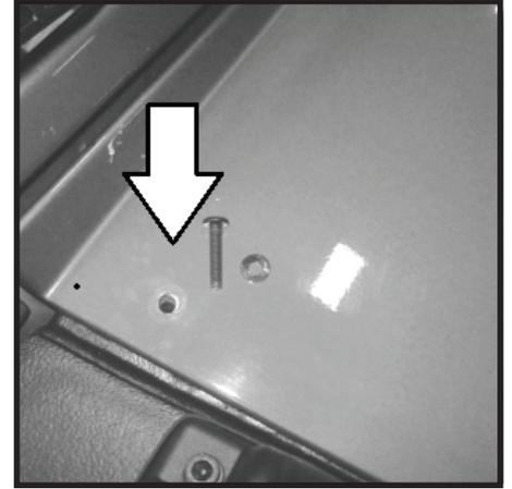
85 - With cowl cover removed tighten "Z"- bracket. Reinstall cowl cover and reinstall drivers side M6 x 20 screws and washers. Reattach center retainer clips removed in step (5).
