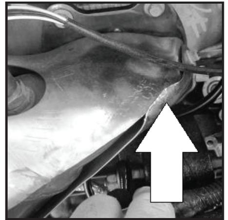
49- Insert aluminum air tube from fire wall forward between shock tower and engine. Front of tube will fit under power steering hard line and to the left of power steering pump. insert mounting tab behind brake bracket. (3.6L) Check heat shield clearance to tube.
