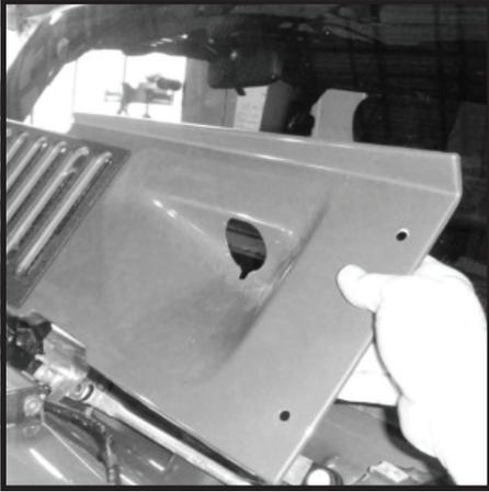
83 - Align driver's side top holes and insert (2) M6 x20 Phillips head screws and washers. Secure but do not tighten.
