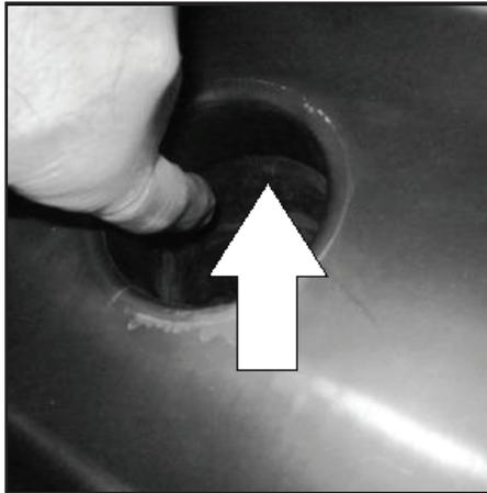
63 - Apply a thin film of sealant around end of aluminum air tube. An excessive amount may cause the elbow to slide off air tube when tightened.
