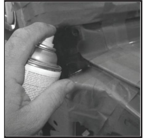
**73** - Make sure painting is done in a well ventilated area. Paint should not be applied in a windy environment. This will insure overspray does not fall onto vehicle.
