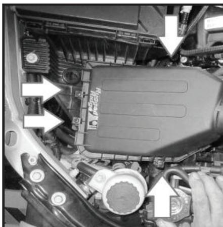
99 - With air box clamps in place and upper air box aligned with new lower air box tighten 3" OE air tube intake clamps at upper air box and intake. Next tighten air box clamps. Confirm upper and lower box are aligned. Tighten radiator 10mm bolts. DO NOT OVER TIGHTEN.
