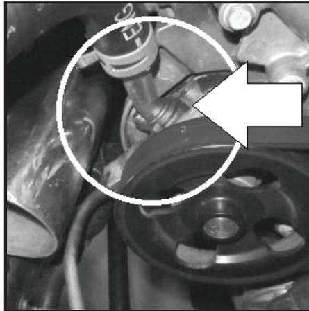
**54-** Place 3" clamps onto both ends of aluminum air tube. Lower clamp should have screw face at the bottom of the tube facing outward as shown. The upper clamp should have screw face at the top facing outward.
