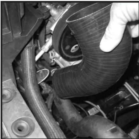
**56-** Place new lower air box onto elbow making sure elbow is fully seated to air box inlet. Air box should rest within 1/8" of rubber grommets.
