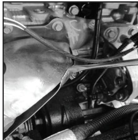
51 - With adjustments made insert tube and place mounting tab behind brake line mounting bracket. Secure 10mm bolt but do not tighten at this time. Final adjustment of air tube will be done later.
