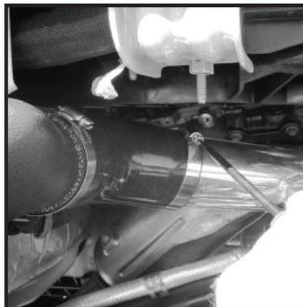
**93** - Slide 3/8" drain hose and 3/8" clamp to bottom of snorkel body.
