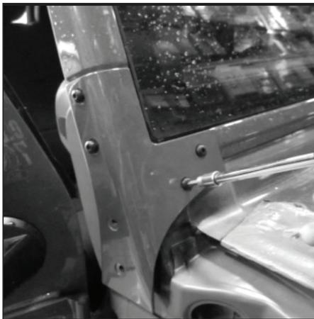
**75** - If used, windshield light mounting brackets should be installed at this time. NOTE: the snorkel system has been designed to work with most Rugged Ridge components. Rugged Ridge cannot guarantee that other manufactures components will work or clear the XHD snorkel system.
