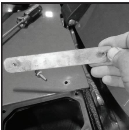
87 - Slide nut plate under snorkel body as shown. Working from engine compartment align mounting holes. Start one M6 Phillips head screw to hold in place.
