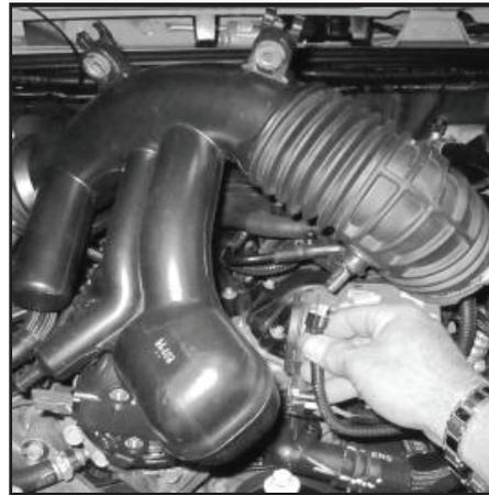
**45 -** Disconnect factory air intake tube from upper air box, place to the side. Upper air box will be reused. Do Not Discard.
