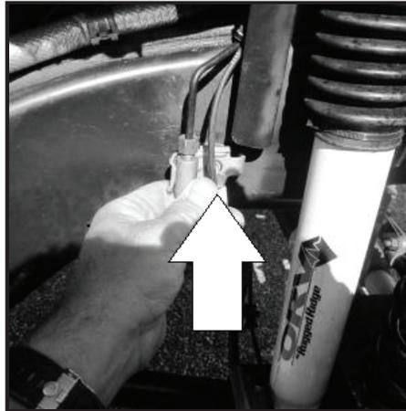
48 - (NOTE: 3.6L Only) Inspect exhaust manifold heat shield. Shield may need to be clearanced to allow aluminum air tube to fit correctly. Fold heat shield over as shown. Clearance until air tube no longer makes contact.
