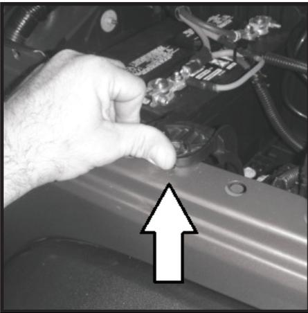
**17** - Top of rear fender will need to be lifted and cleared from inner mounting frame. If needed a small flat head screw driver can be used. Care must be taken to not bend the fender. Slide head of screw driver between the fender and frame. Carefully lift and pull fender too clear.
