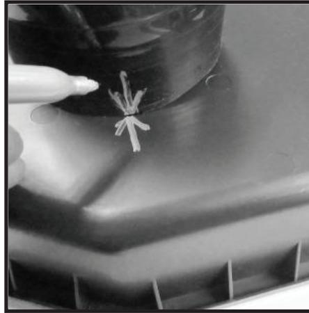
60 - Apply a small amount of quality sealant to the inside of each end. Spread sealant evenly. A thin layer is all that will be needed for the inside to seal correctly. Too much sealant can act like a lubricant during final assemble and cause tube to slide off inlet.
