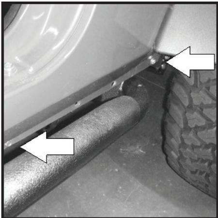
**104** - Secure top of fender to inner fender frame. Battery tray support will need to be lifted to allow fender to slide under support.
