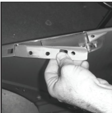
**32** - Carefully trim extra metal from inner antenna support bracket as shown. DO NOT cut too deep or damage to outer fender may result. A Dremmel tool with a cut off wheel is recommended.
