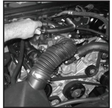
97- For 2012 - Present 3.6L models rotate 3" intake tube back into place and loosely attach to upper air box. Connect crank case hose and wire harness. Loosely start 10mm radiator retainer bolts but do not tighten.
