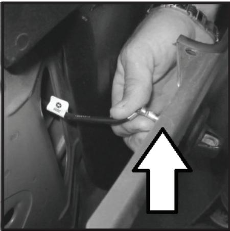
**101** - Slide fender up & over fender support bracket (noted in step (12)). Inspect area around snorkel body. Fender should fit tight to seal but should not be forced to align with fender mounting holes. If fender opening needs to be trimmed for better fit refer to steps (30) through (36).
