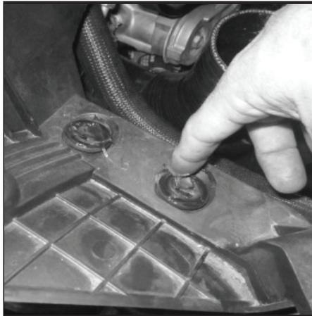
**66** - Apply sealant to corresponding holes on the underside of inner fender mounting plate.
