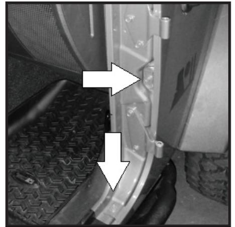
**103** - Align lower fender holes with pinch weld mounting holes. Reuse bolts removed in step (15). Secure bolts but do not tighten at this time.
