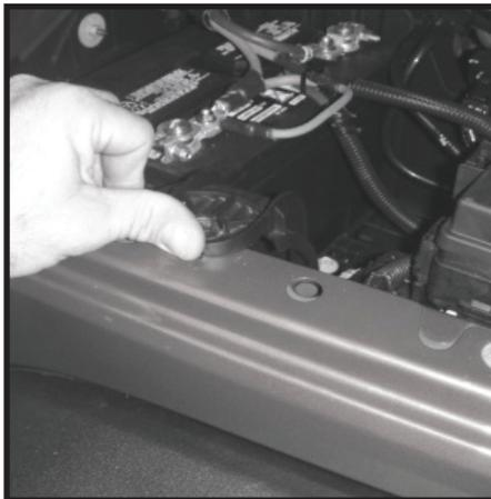
**105** - Reinstall all remaining bolts removed in steps (8) through (13). Secure all bolts but do not tighten at this time.
