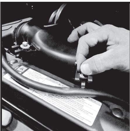
98- Adjust (4) air box sealing clamps full open. Clamps are designed to slip under lower air box flange and over flange and ribs of upper OE air box. Place clamps as shown (arrows). Secure but do not tighten clamps.
