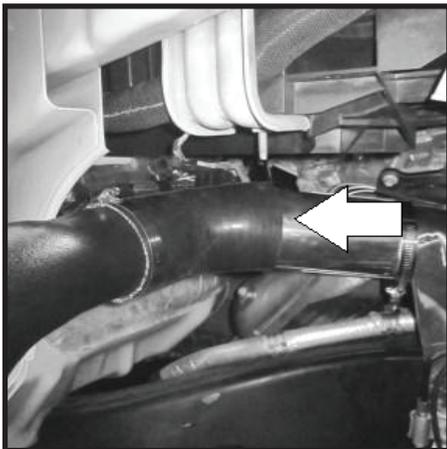
**80** - Snorkel main body should rest in place as shown. Snorkel body should be fitted tight to inner frame. Some vehicles may require the pinch seam (arrow) to be rolled for proper fitment. Check antenna cable position.
