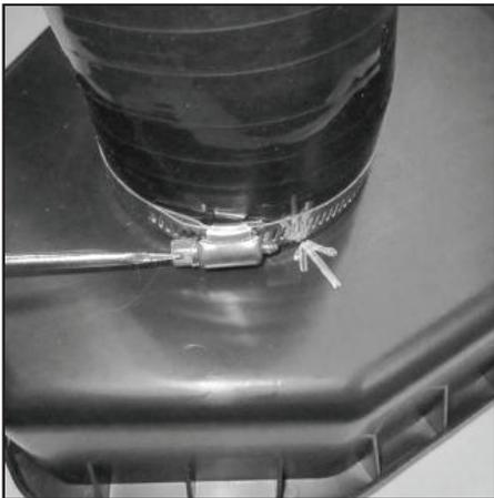
62 - add extra sealant to the inside lip of lower air box inlet and elbow as shown. Extra sealant can also be added to the outside as well.
