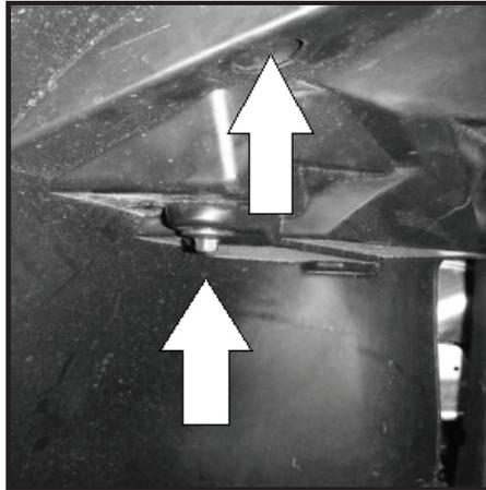
12 - Remove top fender support bolt.
