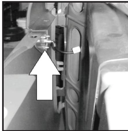
**21** - Carefully lift fender up and away from vehicle. Watch front grill and inner door bolts as fender is removed. Fender must be raised and slid over inner fender support bracket noted in step 12.
