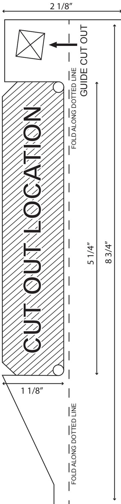
Cut out template using scissors or X-ATCO blade. The template is a (1:1) scale guide for cutting top of passenger side (LH) fender.
