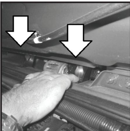
86 - Locate cowl nut plate. Nut plate is used to secure cowl cover and snorkel body to "Z" bracket.
