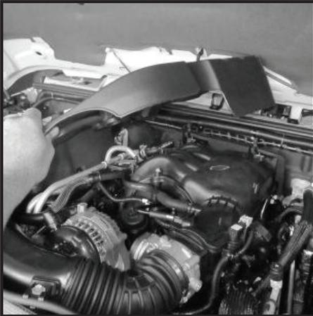
**41 -** Unlatch upper air box from lower air box. Remove factory air filter and set to the side. Filter can be reused if clean. A high flow aftermarket air filter is recommended for use with snorkel.
