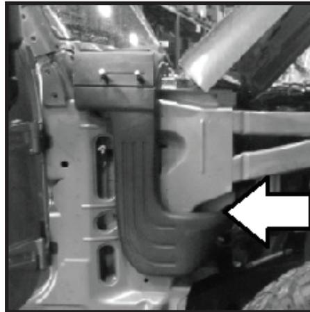
**81** - Inspect "Z"-bracket to snorkel alignment. Adjust snorkel body and "Z"-bracket to align mounting holes. If needed "Z"-bracket can be adjusted (bent) to align all holes.
