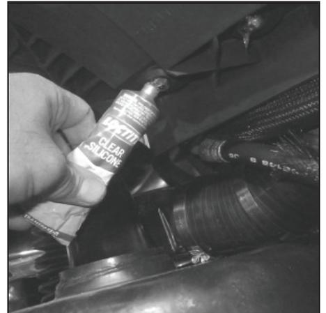
**67** - Reinstall lower air box and 90 deg elbow. Slide elbow over aluminum air tube. Apply extra sealant around outer edge of the elbow and air tube. Slide 3" clamp over elbow but do not tighten at this time.
