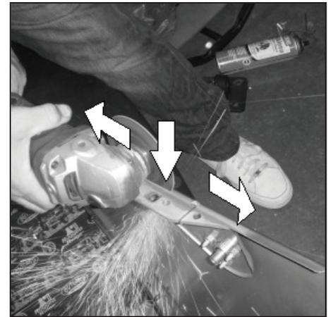
**31** - Allow steel to cool before touching. Remove cut section from fender. Care should be taken when handling rough cut steel.
