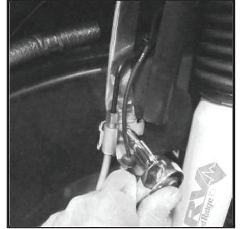
**91** - (Note: 3.6L Only) Tube can be adjusted if additional clearance to heat shield is needed. Grab tube and bend as needed. Make sure lower section of air tube still clears power steering pump and hose (arrows).
