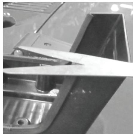
111 - Rest lower intake onto snorkel body as shown. lower (long) M6 caps head bolts will be started first. Starting front lower bolts first allows the intake to be popped into place over the main body intake.
