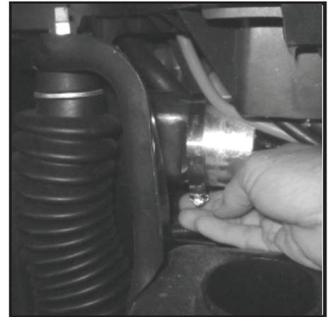
**55-** Place 90 degree silicone elbow onto aluminum air tube. **DO NOT** install 3" clamp. Test fit of lower air box will be needed. Elbow will be removed prior to final assemble.
