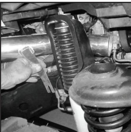
50 - (NOTE: 3.6L Only) Remove air tube and make adjustments to heat shield as needed Upper and lower sections of heat shield can be rolled over as shown. A hammer and flat head screw driver can be used to make adjustments.
