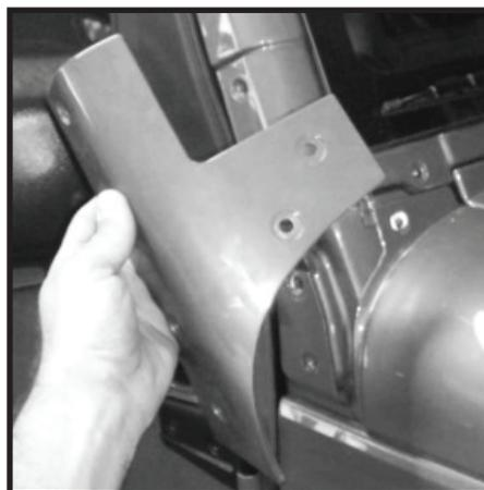
**3** - Remove the (4) cowl screws. A T-30 Screw driver or socket will be required.
