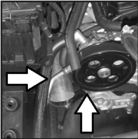
**53-** (Note: 3.8L & 3.6L) **DO NOT** pull or grab the low pressure power steering return line. If line is pulled or forced O-ring seal can be damaged. (3.6L shown).
