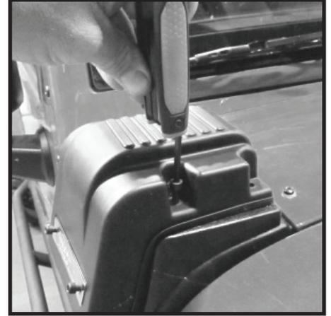
**115** - With intake secure pull outer edge of "U" gasket away from intake until gasket rest flat against side of intake.
