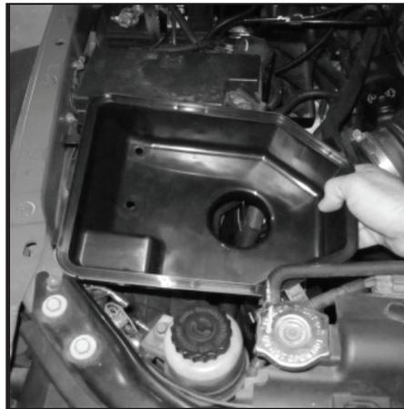
**57 -** If air box does not fit within 1/8" of rubber retainer grommets the top of the silicone air tube will need to be trimmed. Remove air box and elbow. If air box fits correctly proceed to step (59).
