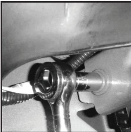
14 - Loosen inner door fender bolts. Do not remove. Allow enough clearance for fender to slide out easily. Notice: If door remains installed bolts should be removed to avoid damage to vehicle if door is closed.
