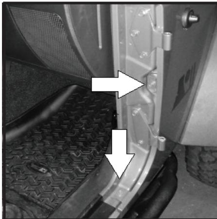
15 - Remove lower pinch weld fender bolts. Note location of bolts. Bolts will be reused. NOTICE: On some models rock rails or side steps will need to be removed before bolts can be accessed.
