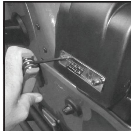
**117** - Reinstall antenna mast.
