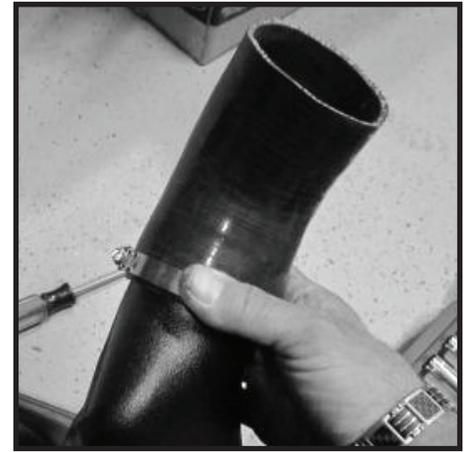
**79** - Add a bead of sealant to the upper section of air tube (arrow). Slip main snorkel body and coupling over air tube as shown. Slide 3" clamp over 45 deg elbow but Do Not tighten.
