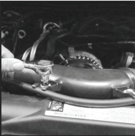
**44 -** Disconnect air tube from air box and intake. place to the side. Sensor wire may need to be disconnected. (3.6L shown)
