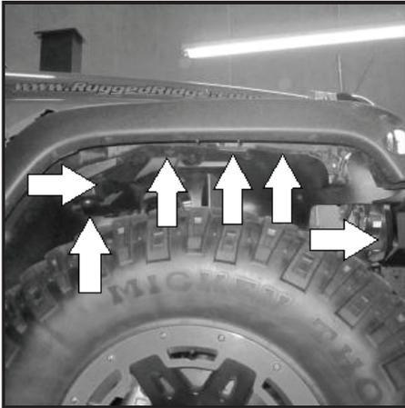
11 - Following four images show locations of key inner fender bolts. Rear inner bolt may be recessed under inner fender liner. See arrow for bolt location.
