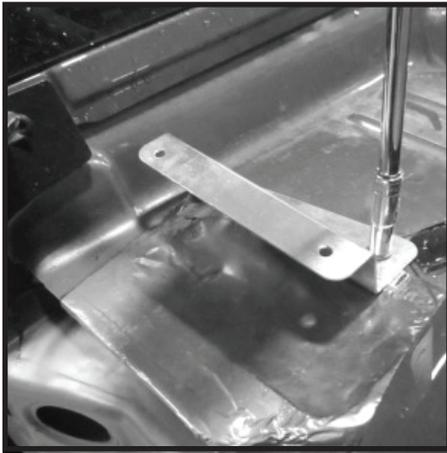
**77** - Dry fit main body, elbow and air tube before applying sealant. If all parts line up apply a thin bead of sealant around the lower section of the snorkel main body. Spread sealant evenly around the outside of the outlet. A thin layer will insure a tight seal.
