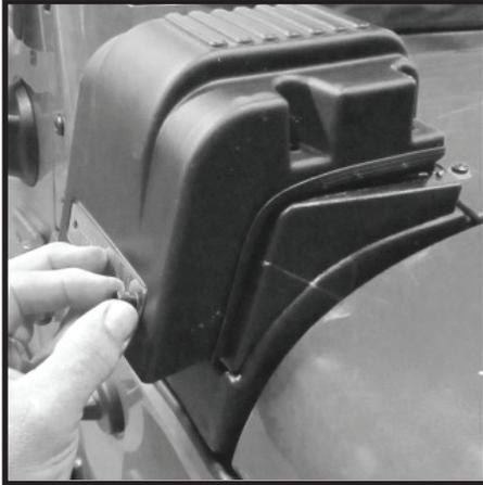
**113** - Press top of intake down onto snorkel body. Intake will fit over top front of main body intake and pop over the rear of intake as shown.
