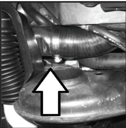
**68** - Insert (2) M8 x 35 bolts with (2) M8 flat washers through lower air box mounting holes and rubber grommets. Apply a small amount of sealant to washers.
