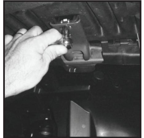
13 - Remove front inner bolt. Bolt is located under inner liner just behind front grill.
