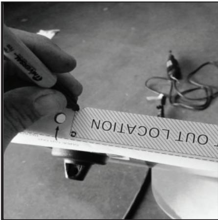
**29**- With guide holes marked and guide holes drawn drill 1/8" centering holes into fender. Use a 7/32" drill bit to enlarge 1/8" guide holes.
