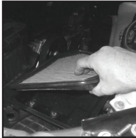
96 - For 2007- 2011 3.8L models Reinstall factory upper air box removed in step (41). Connect crank case vent hose and rotate 3" intake hose back onto upper air box. Reconnect sensor wire harness. tighten clamps and proceed to step (99).
